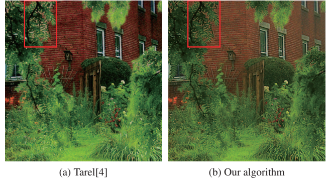
Fig. 3. Comparison with Tarel’s method. (a) Restoration result by [4] for the hazy image Figure 2(a). (b) The result of our approach. Note that in the red rectangle region, due to sharp variations in depth, [4] can not process it well.
